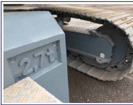
Undercarriage ballast 2,750 kg (x2)
